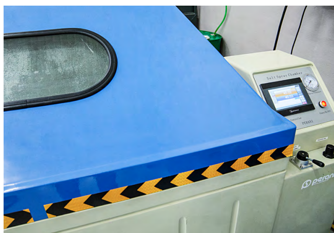
Salt spray test chamber: tests are carried out to the UNI 9227 standard, and in compliance with the specific requirements of the customer.
